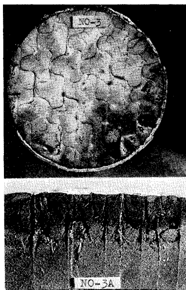
Fig. 9 Post-test appearance of EAS-3560 after simulated 2-pass, high-drag heating.
